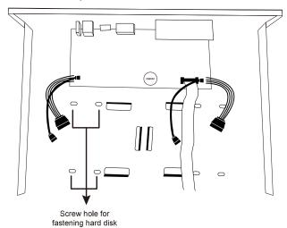
Step2: Get a compatible hard disk. With the PCB side facing down, find the screw holes on the DVR base, and place the hard disk in the DVR.
