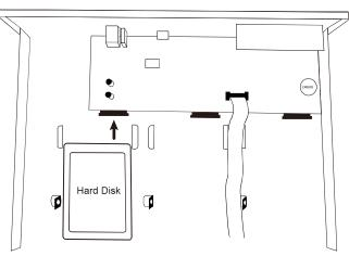
Step3: Fasten the hard disk to the bracket by securing the screw on the bracket.
